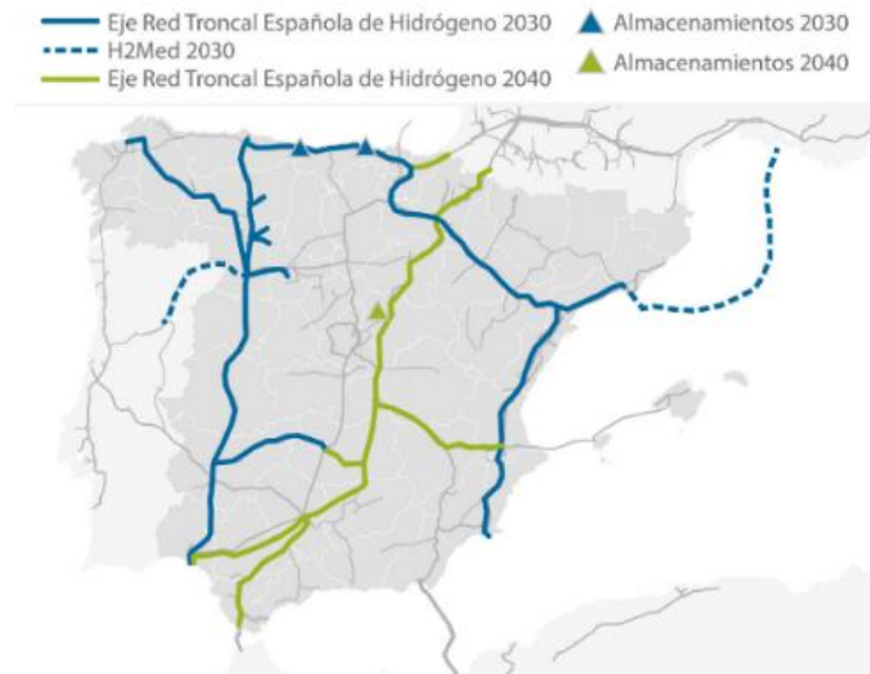
Figure 45. Proposal for basic hydrogen infrastructure proposed by Enagás for Spain in 2030 and 2040. Source: Enagás
