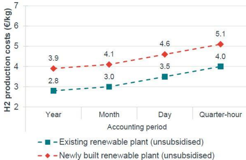
Figure: H 2 -production costs in different accounting periods for existing and new plants (example: combination of PV/wind)
